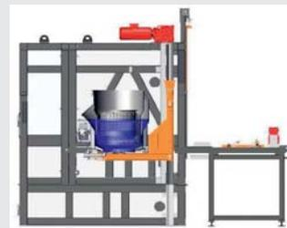
*During the coating process, the product is dipped into the coating media and rotated slowly. The rotation speed is adjustable.*
