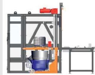
*The basket or rack of parts is automatically indexed into the coating module. Low volume systems can work manually.*
