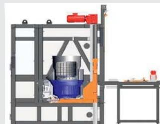
*With or without the WMV paint recovery shell the coating is centrifuged off the parts and returned to the dipping tank. When the paint recovery shield is added to the system up to 5% more of the coating is recovered.*
